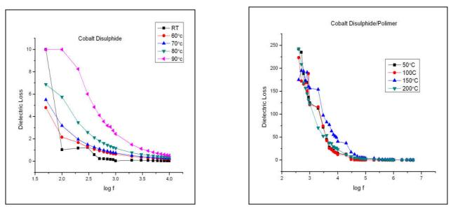
Fig. 6. log f versus Dielectric Loss for pure CoS<sub>2</sub> and CoS<sub>2</sub> in polymer matrix nanoparticles
