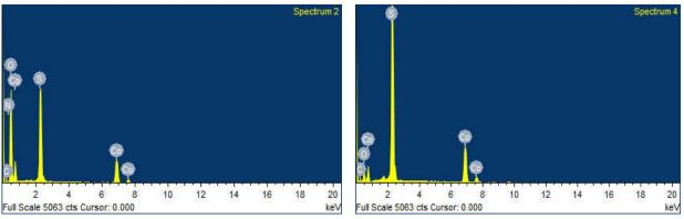
Fig. 4. EDAX spectra of pure CoS<sub>2</sub> and CoS<sub>2</sub> in polymer matrix nanoparticles
