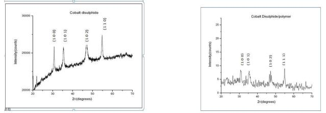
Fig. 1. XRD pattern of pure CoS<sub>2</sub> and CoS<sub>2</sub> in polymer matrix nanoparticles
