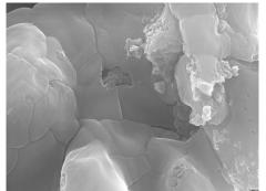
Fig. 3. SEM image of pure  $CoS_2$  and  $CoS_2$  in polymer matrix nanoparticles
