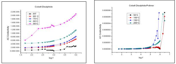
Fig. 7. log f versus Ac conductivity for pure CoS<sub>2</sub> and CoS<sub>2</sub> in polymer matrix nanoparticles
