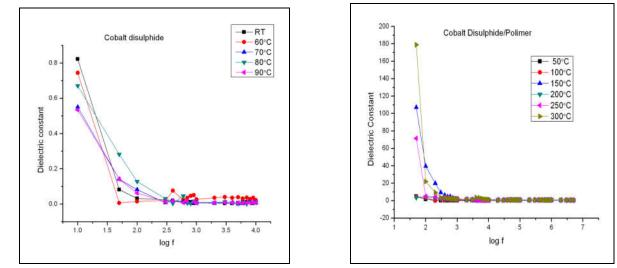
Fig. 5. log f versus Dielectric constant for pure CoS<sub>2</sub> and CoS<sub>2</sub> in polymer matrix nanoparticles
